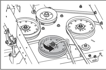
5. Remove the deck belt from the electric clutch on the engine shaft.
