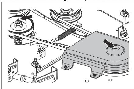
**Note:** Use a grease gun with a rubber hose when you lubricate the cutting deck spindles.
