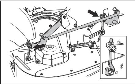
6. Turn the 2 outer blades to align with the cutting deck front to rear.
