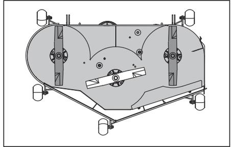
7. Adjust the 2 front bolts until the rear blade tips are set 1/8–3/8 in. / 3.2–9.5 mm higher in the rear than in the front blade tips.
