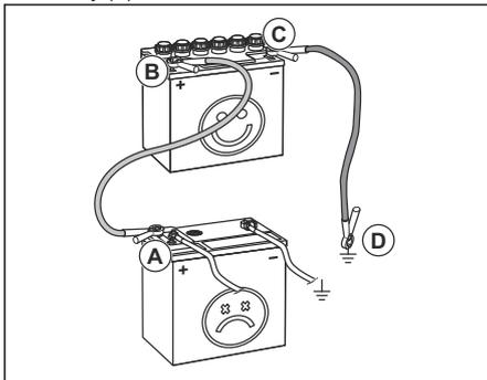
2. Connect the other end of the red cable to the POSITIVE battery terminal (+) on the fully charged battery (B).
