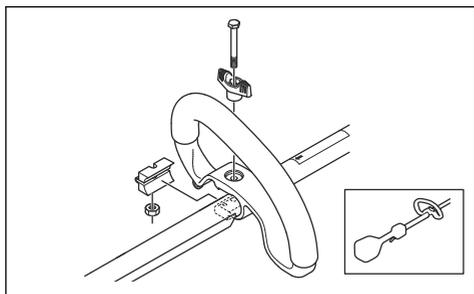
2. Move the spacer into the slot of the loop handle.
