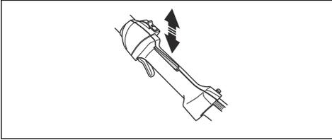
4. Make sure that the throttle control and throttle trigger lockout move freely and that the return springs operate correctly.
