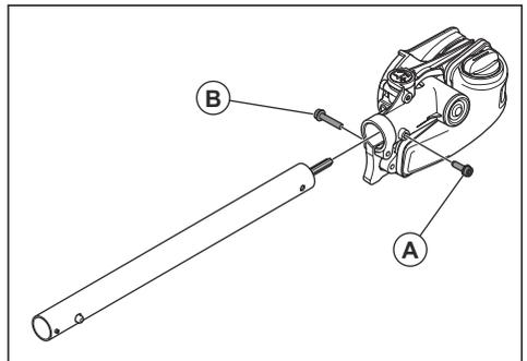
1. Loosen the screw on the cutting head. (A)
