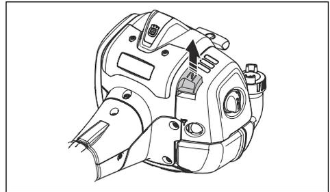
2. Remove the air filter cover and the air filters.
