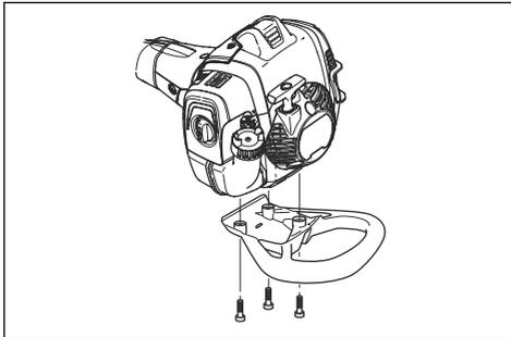
2. Tighten the screws to 30 ft/lbs (4 Nm).
