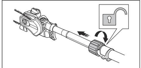
2. Pull out the shaft to the desired length.
