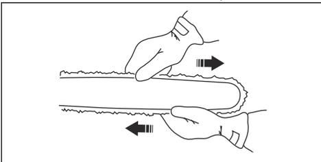
7. When fitting a new chain, the chain tension has to be checked frequently until the chain is run-in. Check the chain tension regularly. A correctly tensioned chain ensures good cutting performance and long life.
