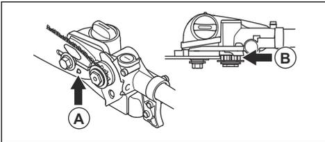
5. Tension the chain by turning the chain tensioning screw clockwise using the combination spanner. The chain should be tensioned until it does not sag from the underside of the bar.
