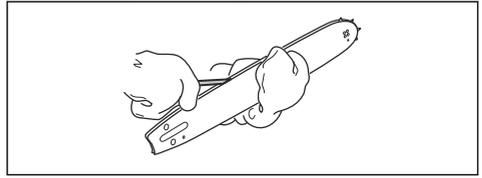
4. Examine the groove in the guide bar for wear. Replace the guide bar if it is necessary.
