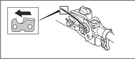
4. Fit the cover and locate the chain adjuster pin (A) in the hole in the bar. Check that the drive links of the chain fit correctly on the drive sprocket (B) and that the chain is in the groove in the bar (C). Tighten the bar nut finger-tight.
