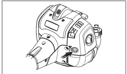
**Note:** It is not necessary to fully fill the bulb.
