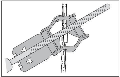
4. Remove material from one side of all the cutting teeth.
