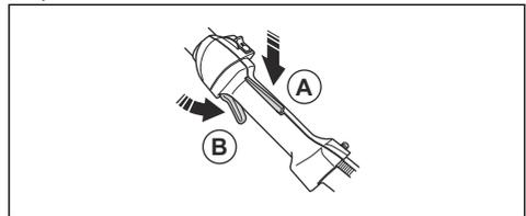
2. Release the throttle trigger lockout and make sure that the throttle control is locked at idle speed.
