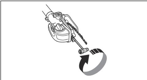
6. The chain is correctly tensioned when it does not sag from the underside of the bar, but can still be turned easily by hand. Hold up the bar tip and tighten the bar nuts with the combination spanner.
