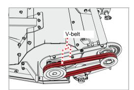
The V-belt unit consists of two narrow V-belts.
