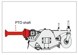
Disconnect the PTO shaft from the carrier vehicle.
