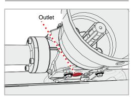
> Place a collection container under the outlet for the waste oil
