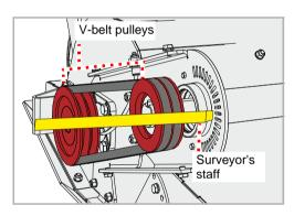
Check the alignment of the V-belt pulleys. Use a surveyor's staff or similar. The surveyor's staff must lie flat on both V-belt pulleys and must be properly aligned.
