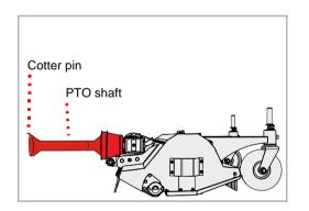
Connect the PTO shaft to the PTO stub shaft of the carrier vehicle. Make sure that the safety split pin on the PTO shaft latches into place.
