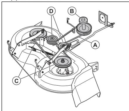
5. Uklonite pogonski remen s remenica vretenaste osovine (C) i remenica napinjača (D).
