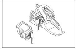
Make sure that the battery has no cracks or other damages.
