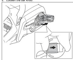
12 2190 - 004 - 12.01.2024 3. Remove the drive sprocket cover and the transportation ring (A).
