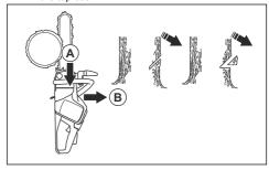
Make sure that the directional cut line is perfectly horizontal and at right angles (90°) to the felling direction. The directional cut line goes through the point where the two directional cuts touch.
