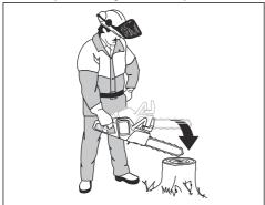
Make sure that the chain brake engages as the guide bar hits the stump.
