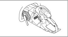
Make sure that the cooling system is not dirty or blocked.
