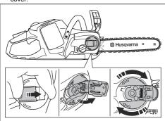
2. Lift the front of the guide bar and turn the chain tensioning wheel. Tighten the saw chain until it is tight against the guide bar.
