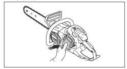
Push and hold the start/stop button until the green LED comes on.
