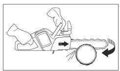
To cut on the push stroke is when you cut with the top of the guide bar. The saw chain pushes the product in the direction of the operator.
