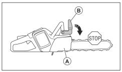
How the chain brake is engaged is in relation to the force of the kickback and position of the product. If you get an intense kickback while the kickback zone is farthest away from you, the chain brake engages by the inertia release. If the kickback is small or the kickback zone is nearer you, the chain brake engages manually by your left hand.
