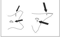
Examine the support flange for cracks. Replace the support flange if it is damaged.
