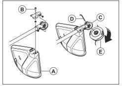
Turn the cutting equipment (E) in the opposite direction from which the cutting equipment rotate.
