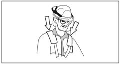
Adjust the harness until the cutting attachment is parallel to the ground.
