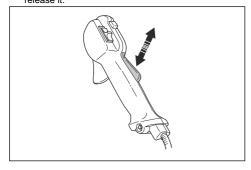
Make sure that the throttle trigger is locked at the idle position when the throttle trigger lockout is released.
