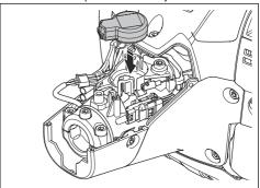
Install the connector to the Husqvarna connectivity device.
