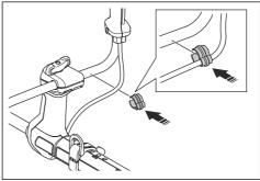
Adjust the handlebar to put the product in a correct work position.
