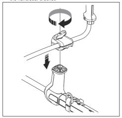
Tighten the handle adjustment knob slightly. Do not tighten the handle adjustment knob fully. 5. Remove the clip from the handlebar. Put the tube into the clip and attach it to the handlebar.
