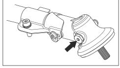
The grease in the bevel gear does not need to be changed unless repairs are carried out.
