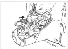
5. Install the plastic cover and tighten the screw.
