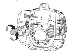
b) Turn the idle speed screw counterclockwise until the cutting attachment stops.
