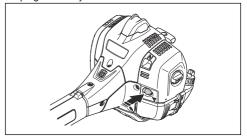
Pull the starter rope handle until the engine starts. Push the throttle trigger slowly to increase the speed gradually.
