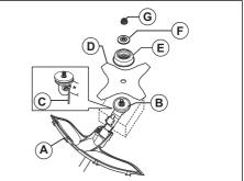
Make sure that the drive disc and support flange engages correctly in the center hole of the grass blade.
