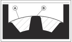
If the grease level is too low fill the bevel gear with Husqvarna bevel gear grease. Fill slowly and turn the drive shaft as you apply the bevel gear grease, stop at the correct level (B).
