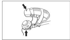
Examine the trimmer head for damages or cracks. Replace the trimmer head if it has been hit or if it has cracks.
