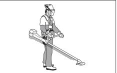
• The product is correctly balanced when the blade is at cutting height near the ground.
