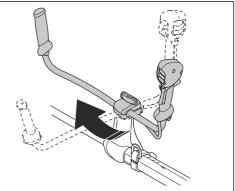
3. Turn the handlebar around the shaft until the handlebar clamp locks into transport position.
