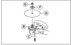
4. Remove the drive disc (B) from the output shaft.
