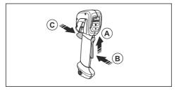
Make sure that the power trigger is locked when the lock is in its initial position.
