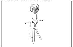
Align the screw hole in the handle with the screw hole in the handlebar.
