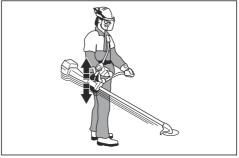
If the operation is to cut grass, let the cutting attachment stay lightly on the ground. Adjust the harness clamp to balance the product correctly.
