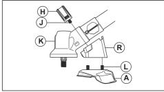
Remove the 2 bolts (J) on the gear housing (K).Remove the holder (R) and the bracket (H).
