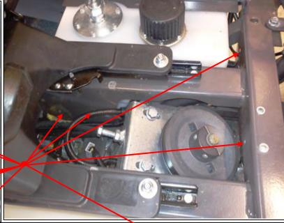
Loosen the original seat by loosening the entire seat console of the machine. Remove these screws. Then loosen the seat of the console.
