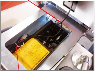
Remove the plastic part and spring in the middle of the connector. Connect the cable to the seat switch from the new seat by insert the spade connectors to the existing contact. Attach the wiring so it can not be trapped or caught in something. Now you can screw the socket head screw as far as it goes. Fold back seat, and now the assembly is complete.
