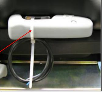
Mount the seat on to the console using 4 pcs M8\*16 mm bolts, and the locknut, mount the seat using the slide rails rear hole. Loosen the cable tie holding the cable to the seatswitch, pull the cable underneath the seat and through the hole in the upper plate of the console, attach the cable with two cable ties in the bottom part of the console, ensure that the cable is attached so it can not be pinched or rubbed off when you fold the seat forward or move the seat back and forth.
