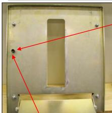
Mount the hexagon bolt in the threaded hole, from below, screw the bolt only about a centimeter trough (if you screw the bolt to the max, you won't be able to mount the seat later on)
