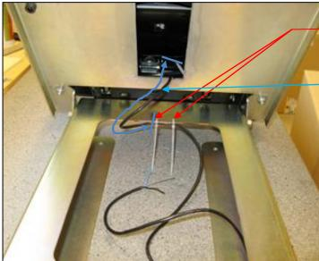
Attach the cable with two of the enclosed cable ties, attach the cable underneath the console so you don't damage the cable when you tip down the seat, as shown on the picture to the left. The cable should measure 24 cm between the cable tie mounted in the seat and the ones mounted on the console.
