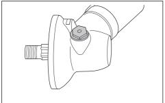
Look into the grease plug hole and turn the drive shaft. The grease level (A) must be in level with the top of the gear cogs (B).
