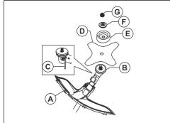
6. Make sure that the drive disc and support flange engages correctly in the centre hole of the grass blade.
