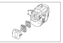
Clean the air filter at an interval of 25 hours, or more regularly if you operate the product in conditions with much dust.
