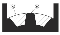
If the grease level is too low fill the bevel gear with Husqvarna bevel gear grease. Fill slowly and turn the drive shaft as you apply the bevel gear grease, stop at the correct level (B).
