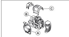
2. Make sure that the cooling system is not dirty or blocked.
