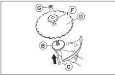
Make sure that you operate the socket wrench in the identified area when you loosen or tighten the saw blade nut.
