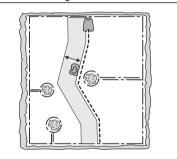
The corridor width is adjusted automatically. Only some times it is necessary to enter manual settings. The corridor width can be set between 0-9. If guide corridor width is set to 0, the product straddles the guide wire. The factory setting is 6 for the boundary wire and 9 for the guide wire.
