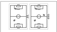
The installation of the boundary wire and charging stations must be made in parallel. Maximum width of the work area is 70 m / 230 ft.
