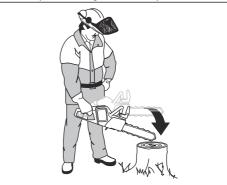
5. Make sure that the chain brake engages as the guide bar hits the stump.
