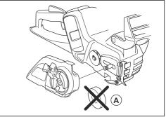
Put the guide bar on top of the bar bolt. Steer the guide bar to its most rear position. Lift the saw chain above the drive sprocket and engage it in the groove on the guide bar. Start on the top edge of the guide bar. 4. Make sure that the edges of the cutting links are turned forward on the top edge of the guide bar.
