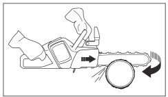
• To cut on the push stroke is when you cut with the top of the guide bar. The saw chain pushes the product in the direction of the operator.
