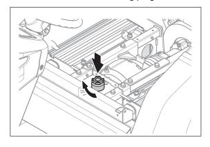
4. Remove the service lid by unscrewing the 2 screws
