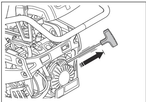
5. Release the starter rope handle to let the starter rope go back.
