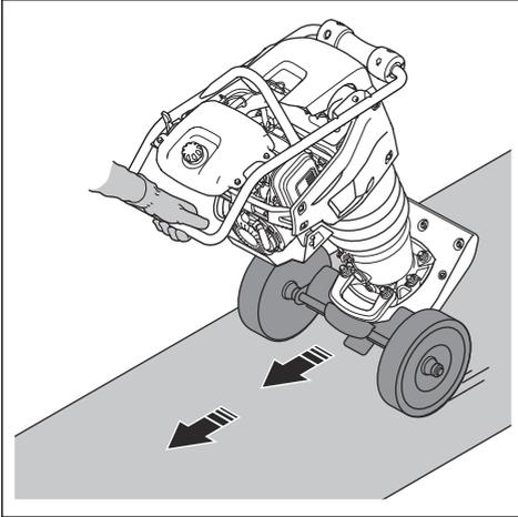
5. Remove the transport device in the opposite sequence.
