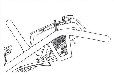
2. If the engine is cold, push the primer bulb 5 times.
