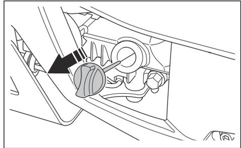
4. Put the dipstick back fully into the oil tank.
