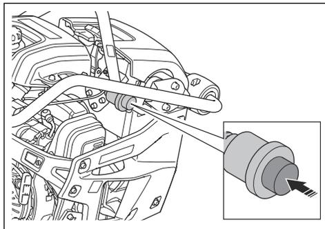
10. Fold the air filter cover down and put the rubber latch back to the locked position of the air filter cover.
