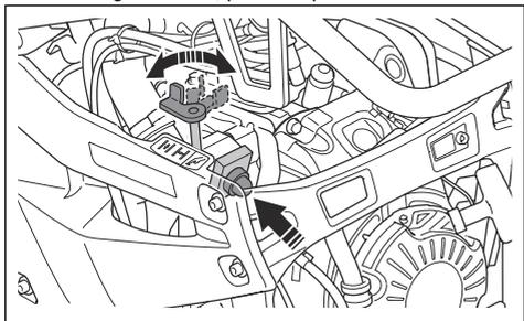
3. Set the choke control in the correct position.
