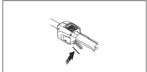
2. Press the power trigger and make sure it returns to its original position when you release it.
