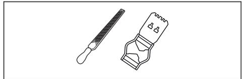
1. Use a flat file and a depth gauge tool to adjust the depth gauge setting. Only use the recommended depth gauge tool to receive the correct depth gauge setting and bevel for the depth gauge.
