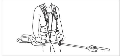
**Note:** The product is correctly balanced when you use minimum hand force to tilt the saw head.
