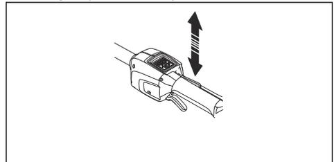
3. Make sure that the power trigger and the lock moves freely and that the return spring works properly.
