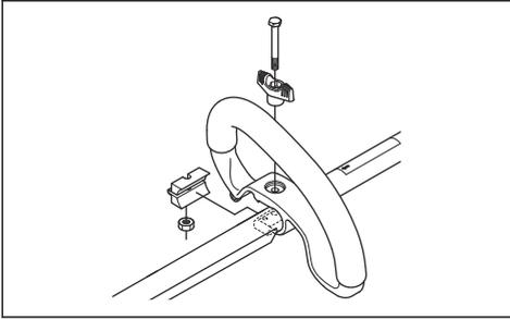
2. Move the spacer into the slot of the loop handle.
