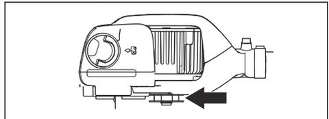
2. Replace the chain drive sprocket if it is worn and moves from side to side on the motor axle.
