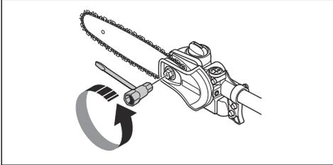
2. Tighten the bar nuts by hand as tightly as you can.
