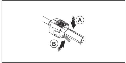
1. Make sure that the power trigger is locked when the lock is in its original position.
