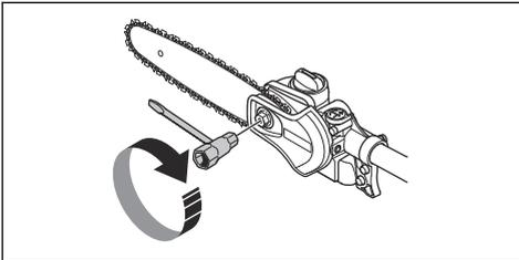
6. Make sure you can pull the saw chain around freely by hand and that it does not hang from the guide bar.
