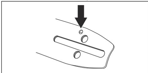
2. Check that the oil channel in the gear housing is clean. Clean if necessary.
