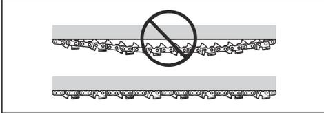
3. Move the file from the inner side of the cutting teeth and out. Decrease the pressure on the pull stroke.
