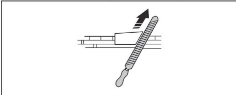
4. Remove filing material on all teeth on one side first.
