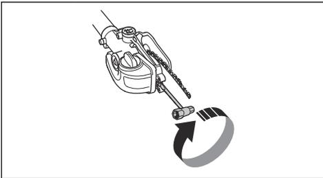
4. Tighten the saw chain until it is tight against the guide bar but still can move easily.
