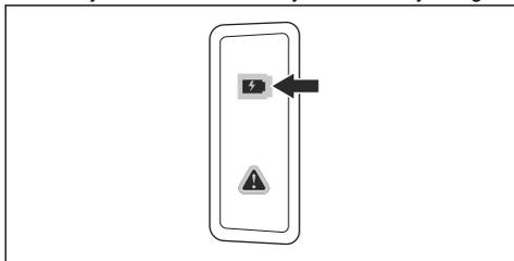
4. When all LEDs on the battery come on, the battery is fully charged.
