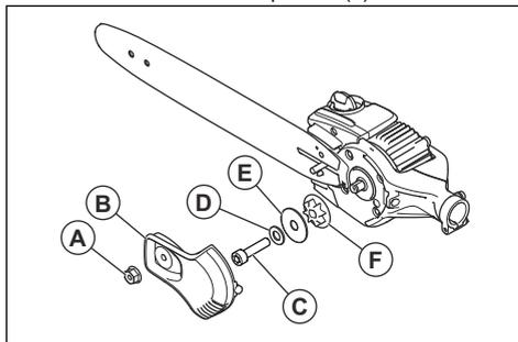
7. Install a new chain drive sprocket.
