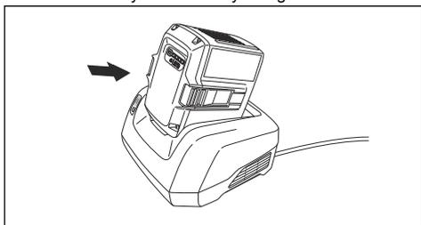
3. Make sure that the green charging light on the battery charger comes on. That means that the battery is connected correctly to the battery charger.
