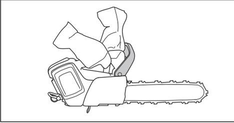
3. Apply full power and tilt your left wrist forward to engage the chain brake.
