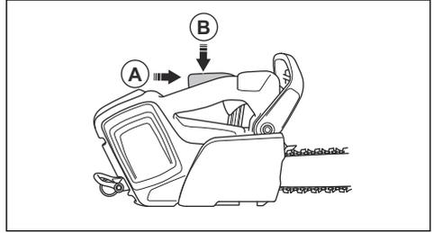
3. Make sure that the power trigger is locked at the idle position when the power trigger lockout is released.
