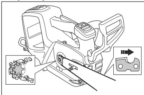
5. Make sure that the edges of the cutters point forward on the top edge of the guide bar.
