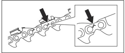
2. Make sure that the saw chain is easy to bend. Replace the saw chain if it is rigid.
