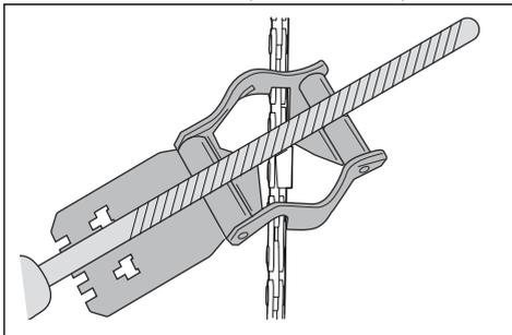
4. Remove material from one side of all the cutting teeth.
