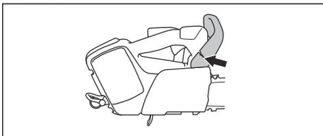
2. Make sure that the front hand guard moves freely and that it is attached safely to the product.
