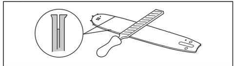
3. Clean the groove in the guide bar.
