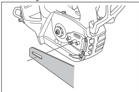
4. Steer the guide bar to its most rear position. Lift the saw chain above the drive sprocket and engage it in the groove on the guide bar. Start on the top edge of the guide bar.
