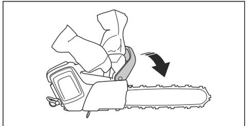
In the felling position you cannot engage the chain brake manually. The chain brake can in this position only be engaged by the inertia release mechanism.
