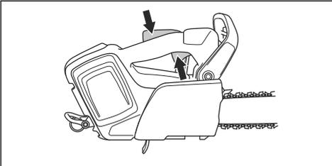
2. Push the power trigger lockout forward (A) and down (B). Hold the power trigger lockout against the handle and make sure that it goes back to its initial position when you release it.
