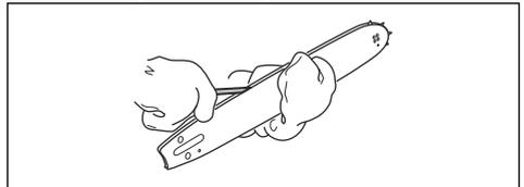
4. Examine the groove in the guide bar for wear. Replace the guide bar if it is necessary.
