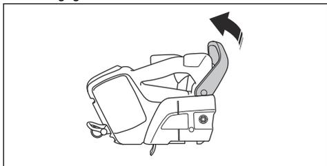
2. Loosen the bar nut. Remove the drive sprocket cover and the transportation ring (A).
