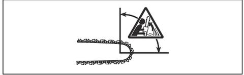
Kickback always occurs in the cutting plane of the guide bar. Usually, the product is thrown against the operator but can also move in a different direction. It is how you use the product when the kickback occurs that causes the direction of the movement.
