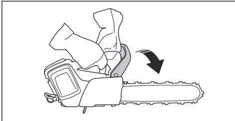
3. Put the battery in the battery holder.
