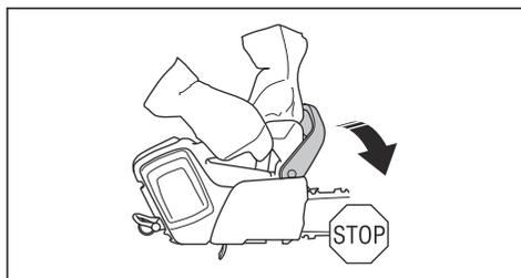
Pull the front hand guard rearward to disengage the chain brake.
