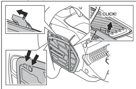
3. Push the air intake cover to the left until the holes align.
