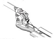
**CAUTION!** The gear housing must not be filled completely with grease. The grease expands as the machine heats up during operation. If the gear housing was completely filled with grease it could damage the seals and lead to leakage of grease.
