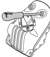
Some mufflers are equipped with a special spark arrester mesh. If your machine has this type of muffler, you should clean the mesh at least once a week. This is best done with a wire brush. A blocked mesh will cause the engine to overheat and may lead to serious damage.
