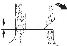
Set the spiked bumper (if one is fitted) just behind the felling hinge. Use full throttle and advance the chain/bar slowly into the tree. Make sure the tree does not start to move in the opposite direction to your intended felling direction. Drive a wedge or breaking bar into the cut as soon as it is deep enough.
