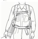
Tighten the side straps so that the pressure is evenly distributed across the shoulders.
