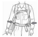
Place the hip strap over the hip and not too far down on the stomach. Tighten the hip strap so that you feel the weight of the blower resting on your hip. Tighten and adjust the breast belt for the best working position.
