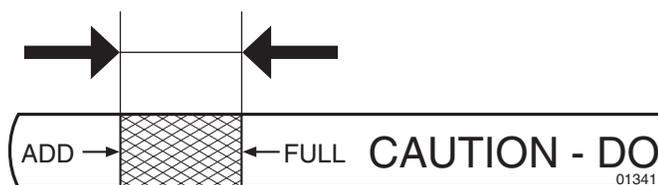
**(GB)** The oil level should lie between the two markings on the oil stick. If more oil is needed add SAE 30 oil to the "FULL" marking. SAE 5W-30 oil should be used during the winter (below freezing point).
