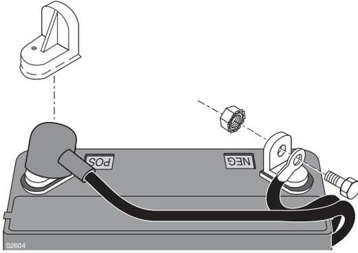
**(GB) ⚠ WARNING:** Positive terminal must be connected first to prevent sparks from accidental grounding.
