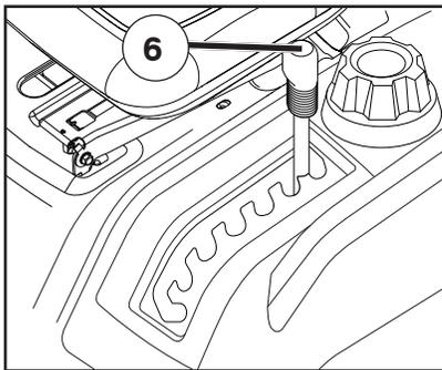
Ⓒ 6. Quick lifting/lowering of the cutting unit
