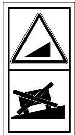
Never use the machine if downwards on slopes with an incline is greater than 10 degrees.
