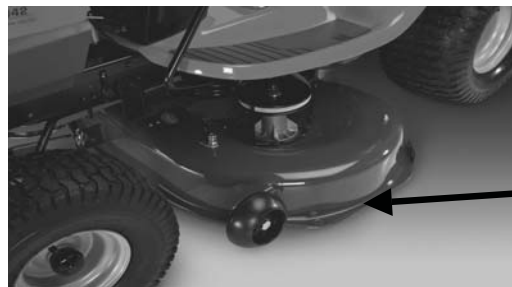
Stamped Deck Shell below, NOT reinforced
