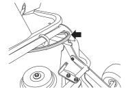
6 Loosen on the cutting height stay and place in the holder.
