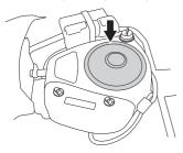
The dipstick should be completely screwed down
