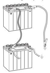
Connect each end of the red cable to the POSITIVE pole
