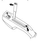
2 Release the clip on the front hood and lift off the fender.
