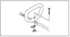
Make sure that the loop handle attaches between the arrows on the shaft
