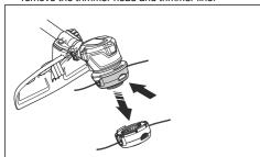
2. Pull out the line chute assembly.
