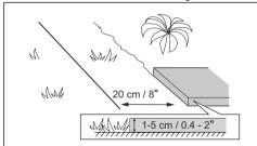
Put the boundary wire 5 cm / 2 in. (D) from an obstacle that is less than 1 cm / 0.4 in. high.
