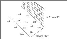
Put the boundary wire 20 cm / 8 in. (C) from an obstacle that is 1-5 cm / 0.4-2 in. high.
