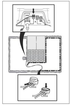
If the indicator lamp now is flashing yellow, then the break is somewhere in the wire between the disconnected end to the point where the new wire is connected (thick black line below). In that case, move the connection for the new wire closer to the disconnected end (roughly at the middle of the suspected wire section) and check again if the indicator lamp is green.
