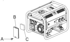
A: BOLT B: AIR FILTER COVER C: FILTER ELEMENT
