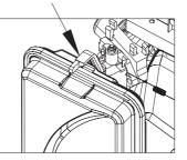
Figure 4 - Choke lever Please note that the choke ON/OFF of 1300 is opposite with this
