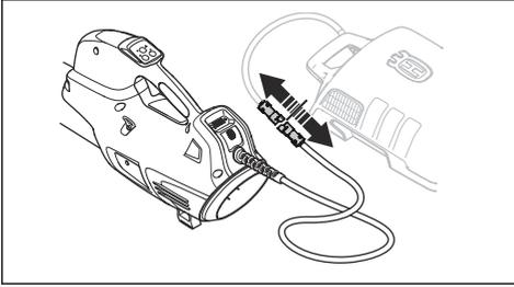
**Note:** If the backpack battery is not used for more than 30 minutes, the backpack battery turns off automatically. To start the backpack battery again, press the start button on the backpack battery.
