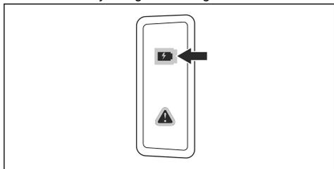
**Note:** The battery will not charge if the battery temperature is more than 50 °C/122 °F. If the temperature is more than 50 °C/122 °F, the battery charger will cool down the battery.
