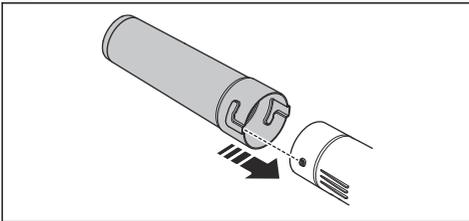
2. Push the blower nozzle in fully and turn the blower nozzle to lock it to the product.
