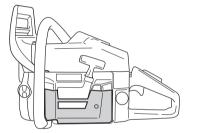
CAUTION! If the special winterising kit has been fitted or any measures have been taken to increase the temperature these changes must be reversed before the machine is used in normal temperature conditions. Otherwise there is a risk of overheating, resulting in severe damage to the engine.
