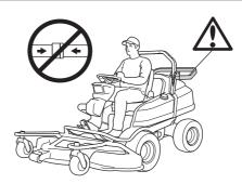
When the safety belt is not used, it must be wrapped around the chair back and tightened.
