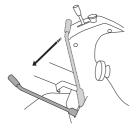
3 Lift the cutting unit with the hydraulic lifting lever.
