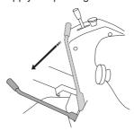
3 Stop the blades by pressing in the control for driving the cutting unit.
