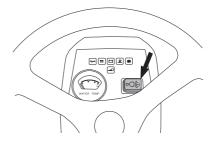
A seat heater or mobile phone charger are examples of articles that can be connected to the power socket.
