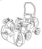
12 Secure the cutting unit with the safety belt, which is stored in the storage compartment under the seat.
