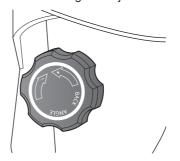
The lumbar support is adjusted with the knob on the left side of seat back.
