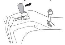
4 Move the throttle control to the MIN. position.
