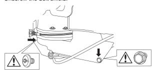
2 Lubricate using a grease gun, 1 nipple from the right-hand side under the engine's lower belt pulley, until grease is forced out.
