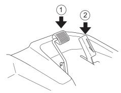
The machine is braked when the forward pedal is released. The reverse pedal can also be used if additional braking power is required.
