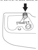
When the choke is engaged a richer fuel and air mixture is fed to the engine, which facilitates starting in the cold.
