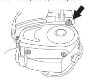
The dipstick should be completely screwed down
