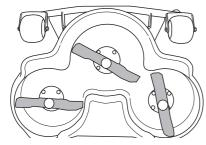
IMPORTANT! One or more unbalanced blades, caused by damage or poor balancing after sharpening, can cause vibrations in the machine.
