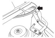
6 Loosen on the cutting height stay and place in the holder.
