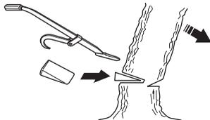
We recommend that you use a bar that is longer than the diameter of the tree, so that you can make the felling cut and directional cuts with single cutting strokes. See instructions under the heading Technical data section to
