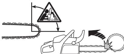
Kickback always occurs in the cutting plane of the bar. Normally the chain saw and bar are thrown backwards and upwards towards the user. However, the chain saw may move in a different direction depending on the way it was being used when the kickback zone of the bar touched the object.
