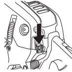
Stop the engine by pushing the start/stop switch down.
