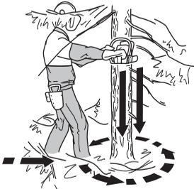
Remove any undergrowth from the base of the tree and check the area for obstacles (stones, branches, holes, etc.) so that you have a clear path of retreat when the tree
