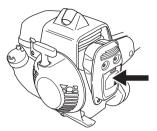
Some mufflers are equipped with a special spark arrestor mesh. If your machine has this type of muffler, you should clean the mesh at least once a week. This is best done with a wire brush.
