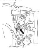
6 To adjust, turn the adjustment screw (B) clockwise and try point 5 again until the carburettor throttle cam bottoms at maximum throttle setting.
