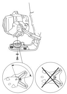
Tighten the nut firmly (approx. 15 Nm) using the combination spanner.
