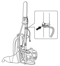
· Hang the flex shaft onto the throttle handle as shown.
