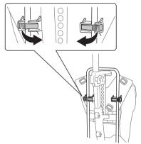
· Loosen the backplate from the frame on one side.
