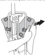
Move the backplate to the desired height and fasten it.
