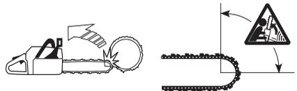
Kickback always occurs in the cutting plane of the bar. Normally the chain saw and bar are thrown backwards and upwards towards the user. However, the chain saw may move in a different direction depending on the way it
