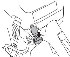
Stop the engine by pushing the start/stop switch down.
