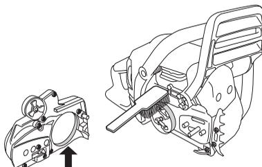
Regularly check that the brake band is at least 0.6 mm (0,024 inch) thick at its thinnest point.
