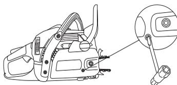
The chain is correctly tensioned when there is no slack on the underside of the bar, and it can still be turned easily by hand. Tighten the bar nut with the combination spanner while holding up the tip of the bar.
