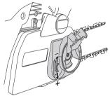
The chain is correctly tensioned when it does not sag from the underside of the bar, but can still be turned easily by hand. Hold up the bar tip and tighten the bar knob by turning the knob clockwise.
