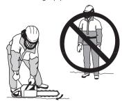
Always hold the saw with both hands. The right hand should be on the rear handle, and the left hand on the front handle. All people, whether right or left handed, should use this grip. Use a firm grip with thumbs and fingers encircling the chain saw handles.
