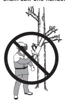
5 You must have a steady stance in order to have full control over the chain saw. Never work standing on a ladder, in a tree or where you do not have firm ground to stand on.
