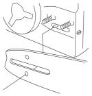
Tension the chain by turning the chain tensioning screw clockwise using the combination spanner. The chain should be tensioned until it does not sag from the underside of the
