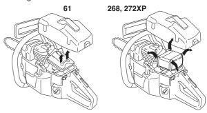
The filter can be cleaned more thoroughly by washing it in water and detergent.
