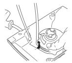
Undo the screw in the centre of the pulley and remove the pulley. Insert and fasten a new starter cord to the pulley. Wind approx. 3 turns of the starter cord onto the pulley. Connect the pulley to the recoil spring so that the end of the spring engages in the pulley. Fit the screw in the centre of the pulley. Insert the starter cord through the hole in the starter housing and the starter handle. Make a secure knot in the end of the starter cord.
