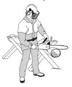
4 Never use the chain saw above shoulder height and try not to cut with the tip of the bar. Never use the chain saw one-handed!
