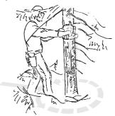
Remove any undergrowth from the base of the tree and check the area for obstacles (stones, branches, holes, etc.) so that you have a clear path of retreat when the tree starts to fall. Your path of retreat should be roughly 135 degrees away from the intended felling direction.
