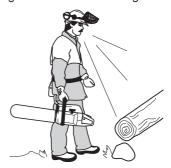
Take great care when cutting a tree that is in tension. A tree that is in tension may spring back to its normal position before or after being cut. If you position yourself incorrectly or make the cut in the wrong place the tree may hit you or the machine and cause you to lose control. Both situations can cause serious personal injury.
