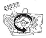
Undo the screw in the centre of the pulley and remove the pulley. Insert and fasten a new starter cord to the pulley.
