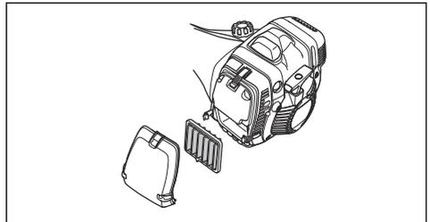
5. Examine and clean the air filter housing with a brush.
