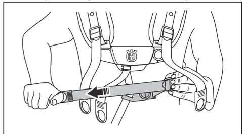
12. Adjust the height of the suspension point. Refer to *Product overview on page 2*. For forestry clearing, the correct height of the suspension is approximately 10 cm/4 in below your hip.
