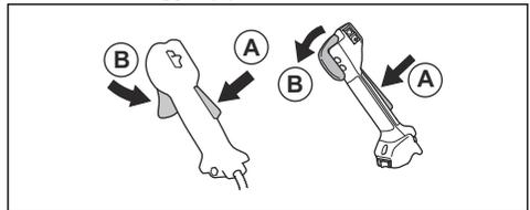
3. Release the handle and make sure that the throttle trigger lockout (A) and the throttle trigger (B) go back to their initial positions.
