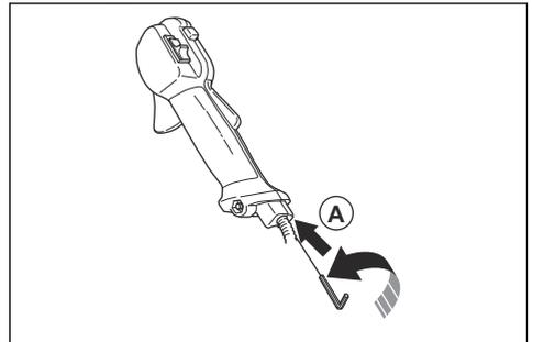
4. If the start throttle speed is more than 6500 rpm, turn the adjuster screw (A) counterclockwise. When the cutting attachment starts to rotate, turn the adjuster screw (A) 1/2 turn.
