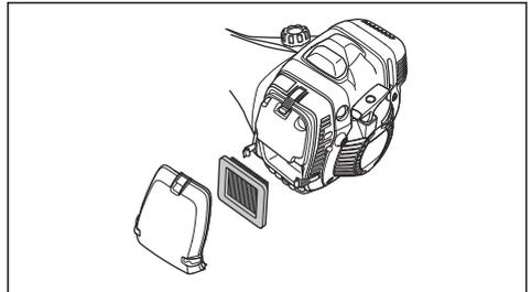
5. Examine and clean the air filter housing with a brush.
