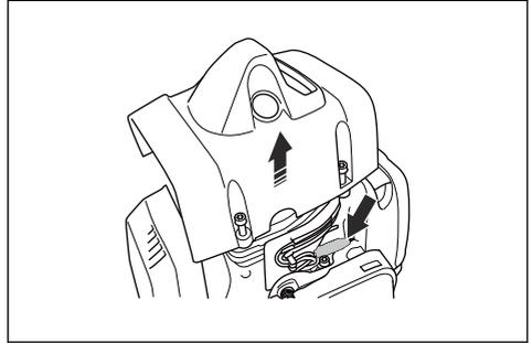
4. Remove the plug on the grease nipple.
