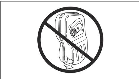
**Note:** The inner surfaces of the muffler contain chemicals that can cause cancer. Be careful not to touch these elements if the muffler is damaged.
