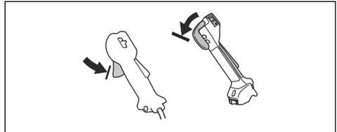
2. Press the throttle trigger lockout (A). Make sure that the throttle trigger (B) is released.
