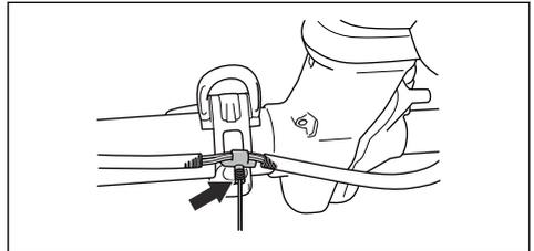
6. Attach the cylinder cover and the protective cover.
