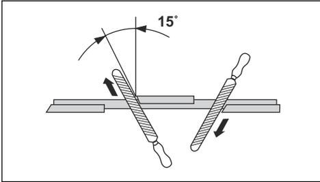
**Note:** Sharpen the edges of the teeth with a flat file if the blade is heavily worn. Continue to sharpen with a round file.
