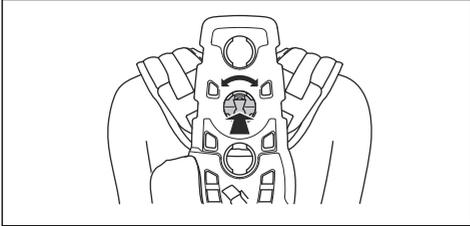
4. Attach the strap (A) in correct position for grass clearing or forestry clearing.
