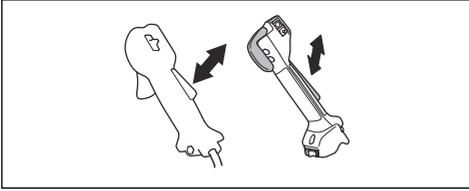
5. Press the throttle trigger (B) and make sure that it goes back to its initial position when you release it.
