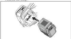
Press the lower part of the battery and push it in as far as it will go into the battery compartment. The battery will lock into position when you hear a click.
