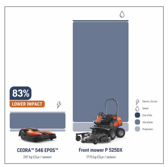
The comparison is made on a scenario of a 30-week cutting season per year. The Lifecycle assessment (LCA) is based on the functional unit of cutting two football pitches (16,000 sqm) of average pitch grass lawn. CEORA is powered by EU electricity grid mix and Husqvarna P 525DX is powered by standard diesel. Result in global warming potential per season (kg  $CO_2e$ /season).
